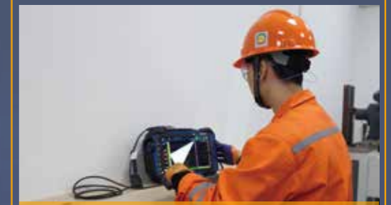
Phased Array Ultrasonic Test (PAUT)
